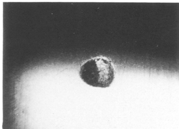
Figure 2 An isolated near-surface bubble, \sim 350 \mu m in size and after mechanical polishing (50 \times ).
